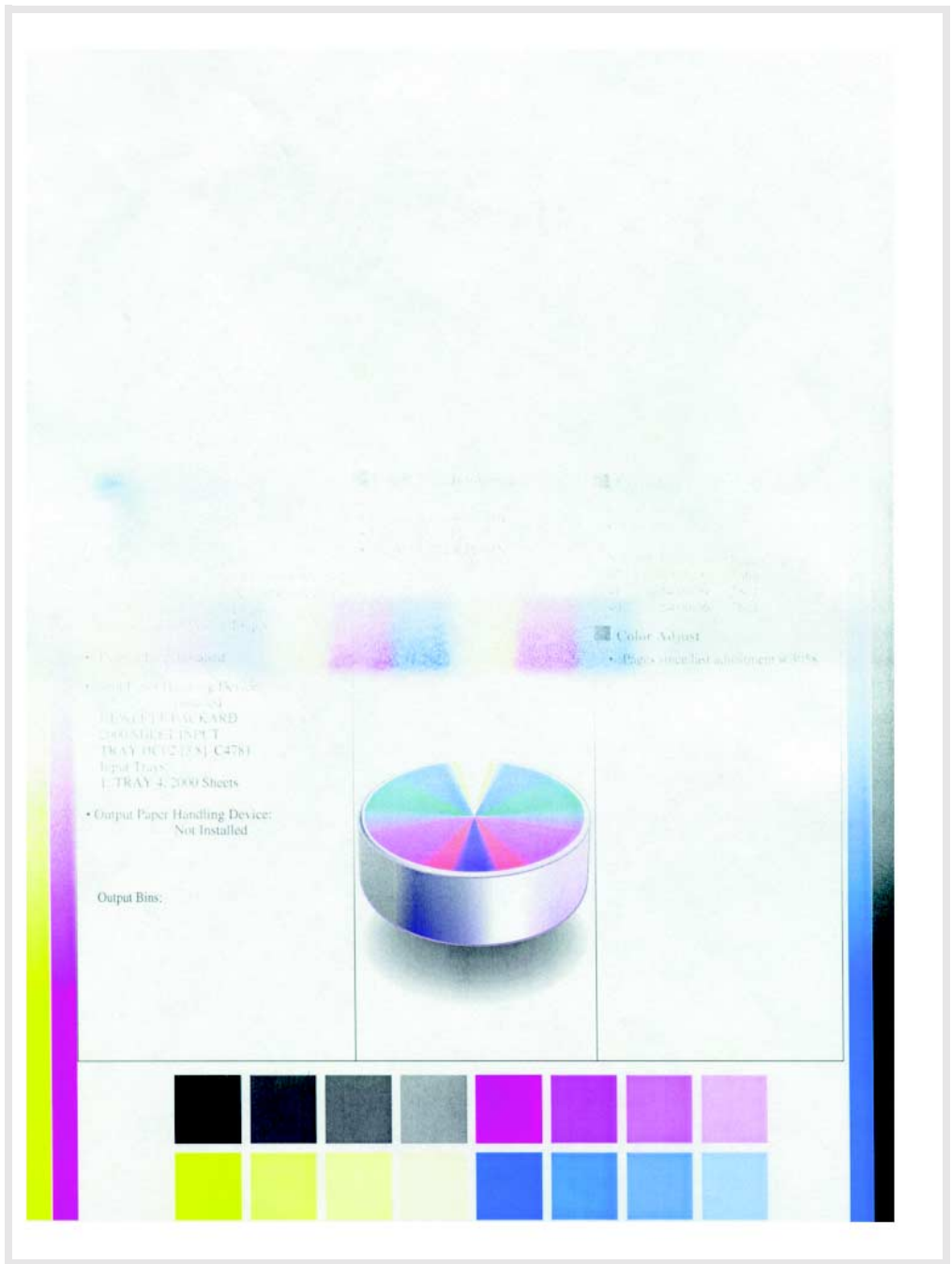
Figure 232. Fading resulting from broken transfer guide
